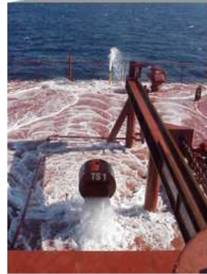
▲ A ship emptying a ballast tank in mid-ocean.
